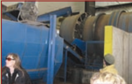
The massive tumbler at the West Yellowstone Compost Facility separates organic material from items destined for the landfill.
