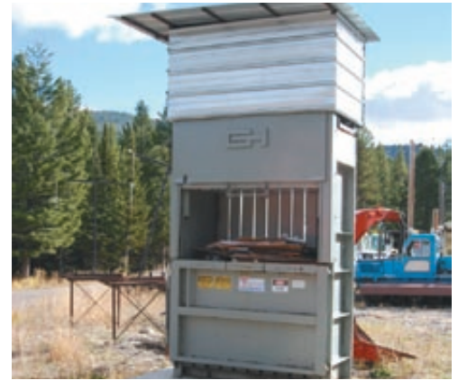
An on-site cardboard crusher helps with recycling efforts.
